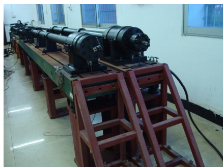
图2 基于 SHPB 的多功能岩石加载试验系统 Fig.2 Multi-function rock loading device based on SHPB
